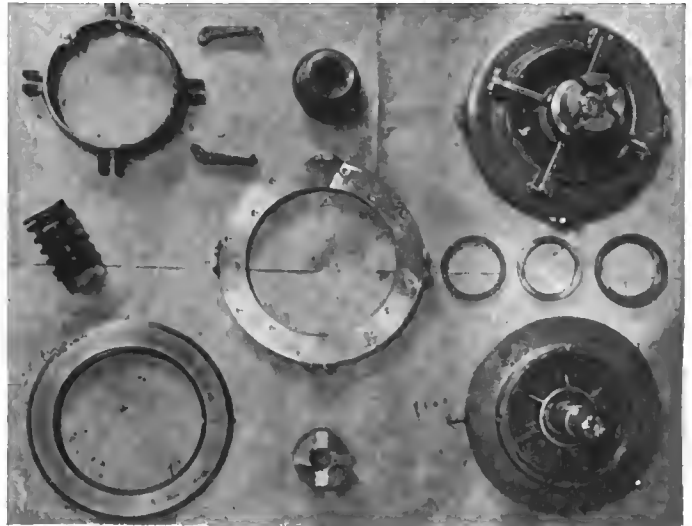
SIMPLE DETAILS OF THE MULTIPLE-DISK CLUTCH.
